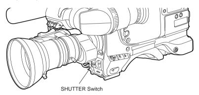
3 Press the SHUTTER switch to the SEL side repeatedly until the desired mode or speed appears. When all modes and speeds can be displayed, the display changes in the order shown below. If the required shutter speeds and modes have been designated beforehand, only the designated speeds or modes appear.
